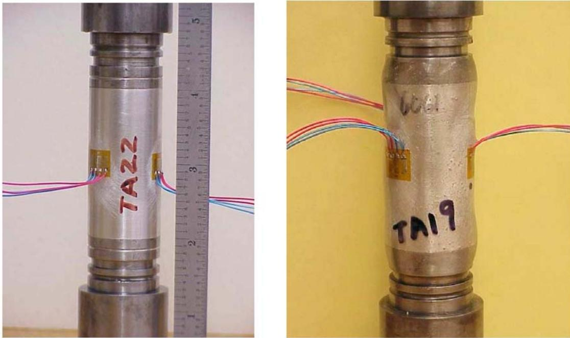
**Figure 5.1.** Strain gaged aluminum specimens
